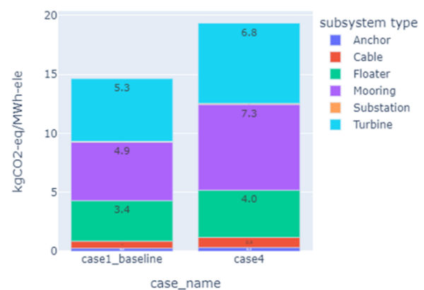
Figure 28: Comparison of carbon intensity by development phase (left) and subsystem (right) for CFA-B-001 and CFA-B-004.
