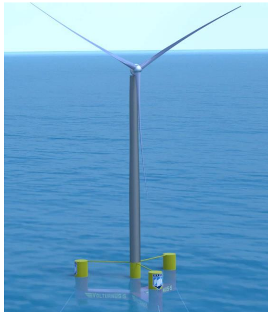
Figure 14: A render of the UMaine VoltunUS-S platform supporting the IEA-15-240-RWT turbine (Allen, et al., 2020).
